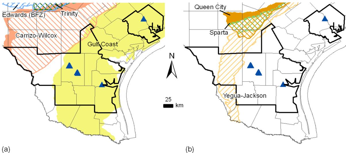
9 Solid indicates a portion of an aquifer that lies at the land surface. Hatched indicates a portion of an aquifer
